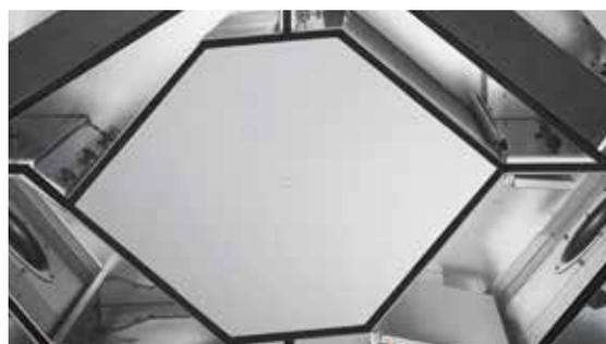
Counterflow heat exchanger can be extracted for cleaning
